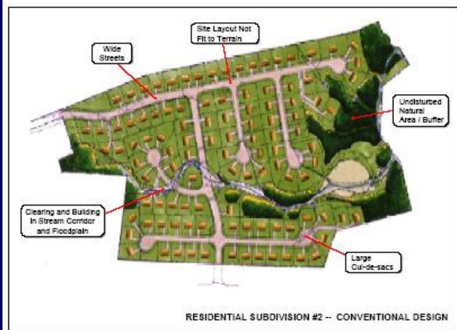
Figure 1.4.3-2 Comparison of a Traditional Residential Subdivision Design (above) with an Innovative Site Plan Developed Using Better Site Design Practices (below).
